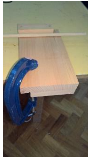
Right handed bench hook clamped to table using G clamp (note that the clamp is on the left to allow space for working)
