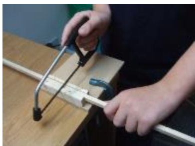
Using a slotted bench hook to cut a right angled cut
