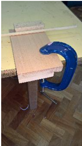
Left handed bench hook clamped to table using G clamp (note that the clamp is on the right to allow space for working)
