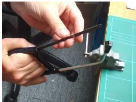
Compressing the frame in a similar way enables you to fit the new blade. The blade is fitted with the teeth facing forward as the saw cuts on the forward stroke.
