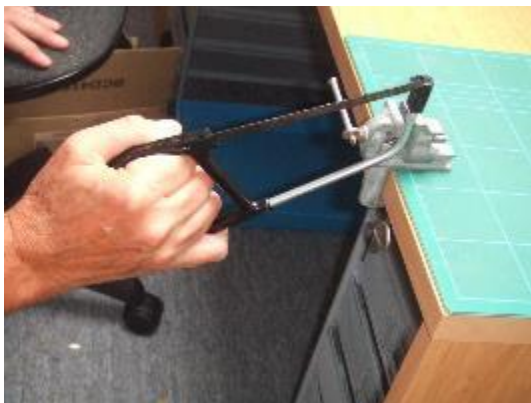
Bending the frame of the saw releases the pins on the blade from notches at each end. The blade can then be removed.
