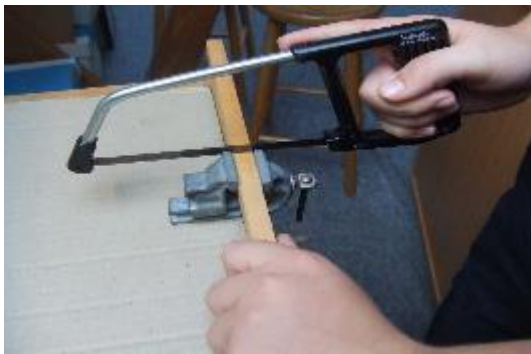
Always saw close to where the vice grips the wood
