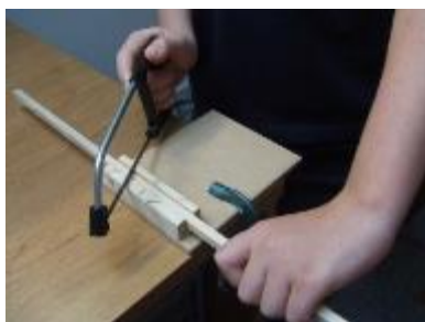
Using a slotted bench hook to cut a 45° cut (mitre)
