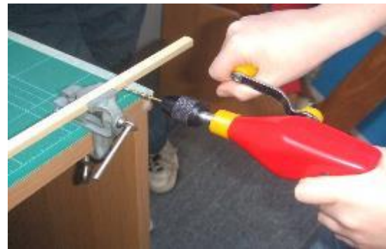
A small vice will hold material steady when drilling. Note the position of the drill close to the vice jaws
