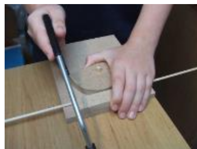
Using a bench hook with a cam to get a better grip on materials.
